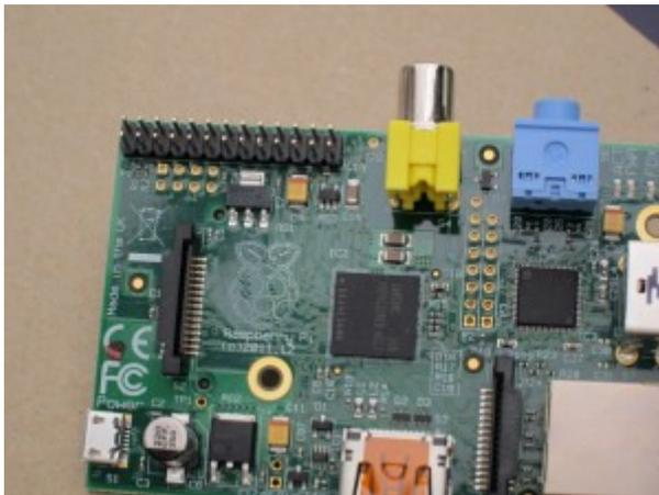
Raspberry Pi P5 connector location before fitting the header – the 8 holes just below the GPIO connector.
