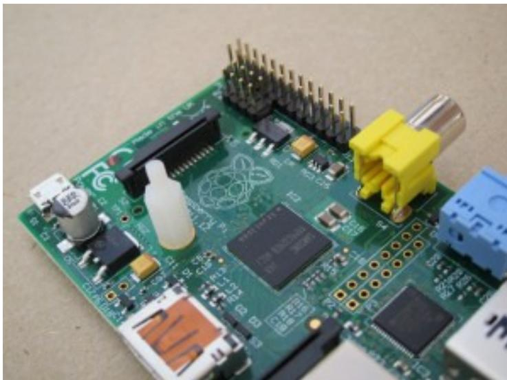
Plug the HiFiBerry into the GPIO and P5 headers while locating onto the standoff. Be careful to make sure all three align before pushing down. It is a snug fit, but does not take much force. Clamp it in place with the nylon nut on top of the standoff.
